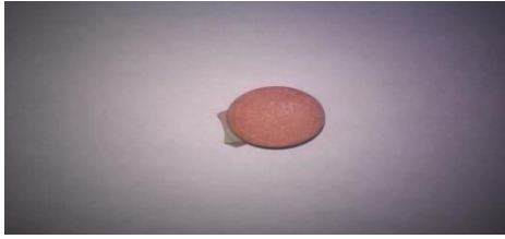
Fig.1.The prepared Polycrystalline LGS pellet
