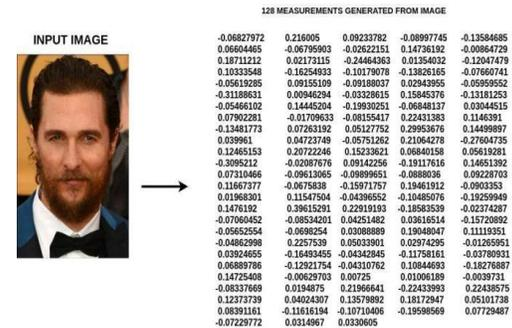
Fig 5: Face Encodings generated from an input image
