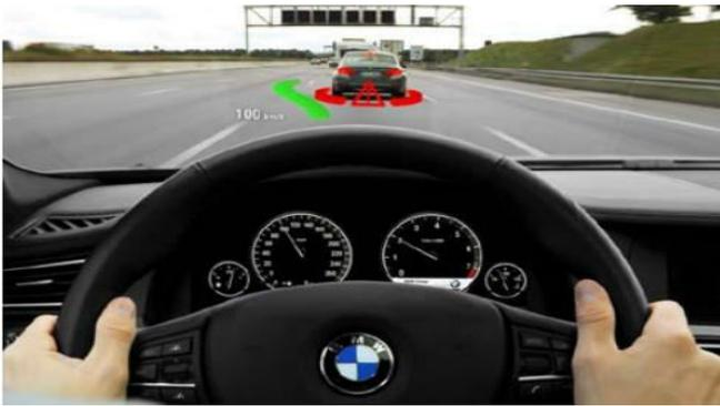
Fig 3: Driver Assistance System for lane departure
