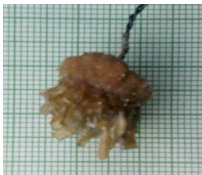
Fig.1. Bunch of orthorhombic Fe doped \text{BiB}_3\text{O}_6 crystals
