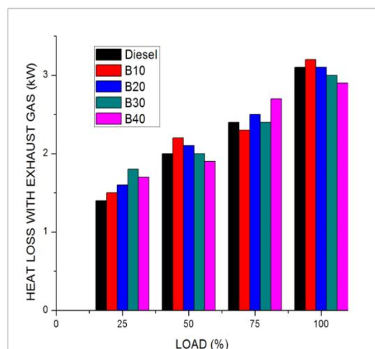
**Fig. 3: Energy loss with exhaust gas at various loads for the tested fuels**
