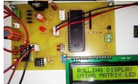
Fig 5: Hardware implementation of digital notice board
