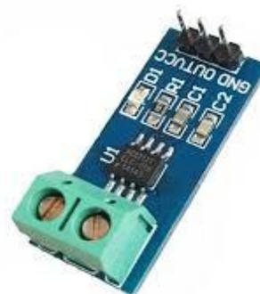
Fig.3. Current Sensor (ACS712)
