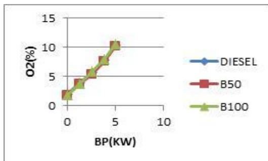
Fig 7: Variation of o2 emission with brake power.
