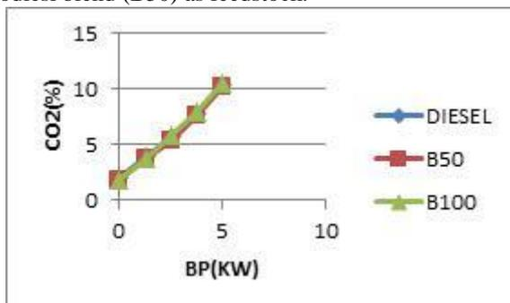
Fig 8: Variation of  $\text{CO}_2$  emission with brake power.
