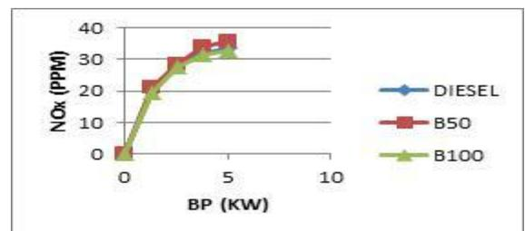
Fig 5 : Variation of NO<sub>x</sub> with brake power.
