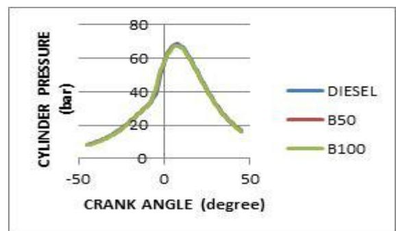
Fig 4: Variation of crank angle with cylinder pressure.
