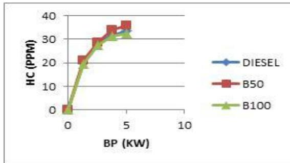
Fig 6: Variation of hydrocarbon emission with brake power.
