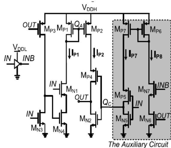
Fig.2. Proposed voltage level shifter.
