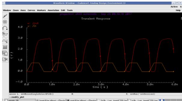
Fig.8. Simulation result of proposed level shifter.
