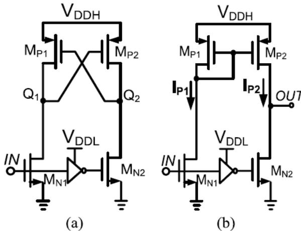
Fig. 1. (a) Conventional voltage level shifter and (b) voltage level shifter with a semi-static current mirror.
