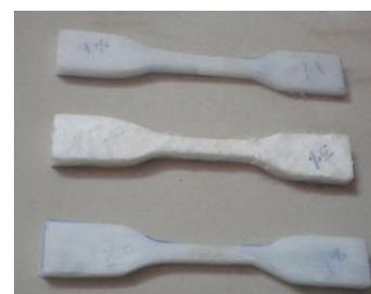
Fig.2. Specimens for Tensile Test
