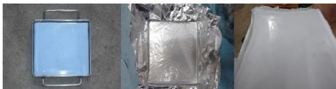
Figure .a) Stainless Steel Die b) Die with aluminum foil c) Syntactic foam
