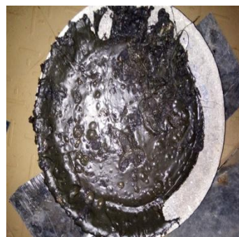
Figure 3: Crude oil extracted during Pyrolysis process
